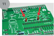
Now for the two capacitors (22pF). These are the two small capacitors. Solder both capacitors to your Fabschoolino.
