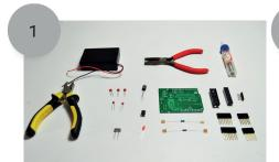
You will need: a soldering iron, solder, a battery holder, the Fabschoolino board (PCB, ATMEGA 328P (ic)), the individual components, and the instructions: Soldering is easy.
