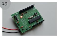
Place three AA batteries in the battery compartment. If everything is working properly, then the LED should flash when you press the reset button. Congratulations, you Fabschoolino is ready to go!
