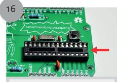
Now take the socket and place it in the holes provided. Solder the socket in place. Note: Make sure the half circle of the socket lines up on the semi-circle on the Fabschoolino.
