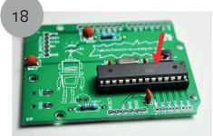
Now place the IC (chip). You just click it into the socket and you don't have to solder. Note: Make sure the half circle of the chip is on the semi-circle of the socket.
