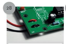
Insert the wire through the second hole. Solder the two wires behind the second hole.
