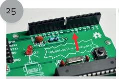
Solder the long header pins. Note: make sure it's correctly inserted and solder it afterwards.
