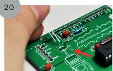
Place the LED in your Fabschoolino. The picture above shows where to insert the long and short legs. Solder it in place.
