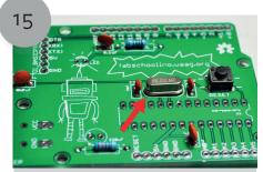
Insert the oscillator into the holes and solder it.
