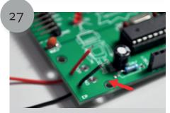
Take your battery holder and run the wires through the first hole as indicated in the picture. The wires should now be pointing out at the top of the Fabschoolino board.
