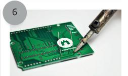
Now you're ready to begin soldering! Hold the soldering iron tip at the foot of the resistor. Hold this for 1 second to warm up the right place on your circuit board.
