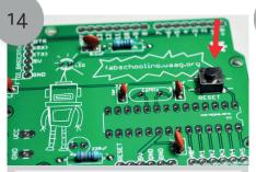
If you've situated the reset button into the holes correctly, you may solder it.
