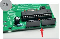
Next, solder the short header pins and cut all 4 feet off the header pins with your cutting tool.
