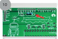
Take the 1k resistor and place it in the Fabschoolino. Solder it in place.
