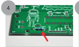
Now take the circuit board and place the resistor in the holes provided.
